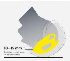
Mips is a low-friction layer inside the helmet. It is intended to reduce the rotational force to the head that is transmitted to the brain at impacts. The system allows for free movement of 10-15mm between the helmet and the head in all directions. The Mips Brain Protection System is a Swedish patented solution based on over 20 years of studies by neurologists, bio-engineers and researchers at the Karolinska Institute and the Royal Institute of Technology.
